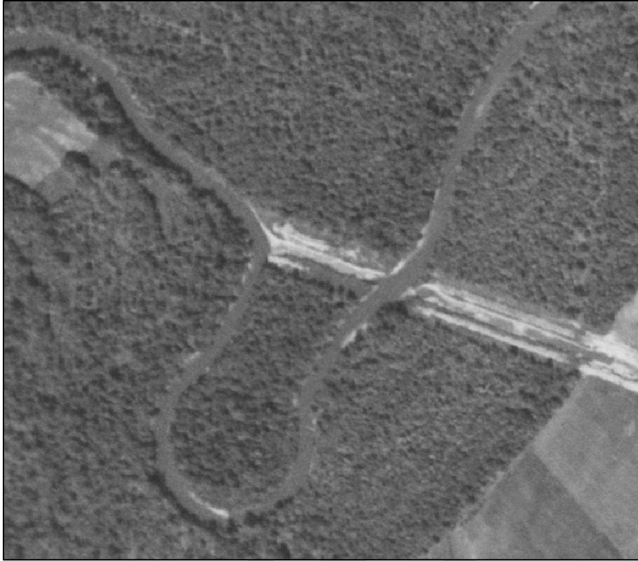
Exhibit 1 Cut-off channel from 1950's. Neuse River still utilized meander as main flow path
